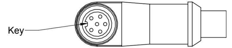
6 Pin Female A-Coded M8 Connector with threaded locking feature - shield passes through the nut
