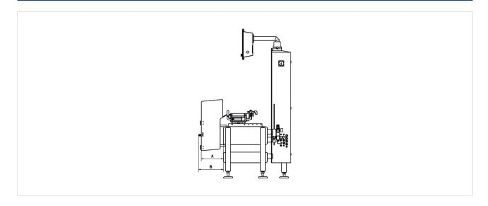
The scale drawing shows Flexus® with a collection container (optional), which is made from plastic or stainless steel – both versions have different dimensions.
